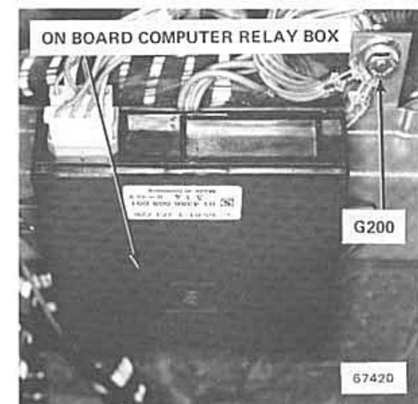
Figure 2 - Under Dash, Left Of Steering Column
