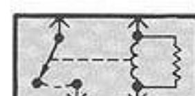
RESISTOR ACROSS COIL IS FOR NOISE SUPPRESSION
